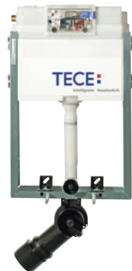
TECEbox brick-wall construction cistern, assembly height 1060 mm, for installation in a bricked curtain wall in front of a solid wall front actuation.
