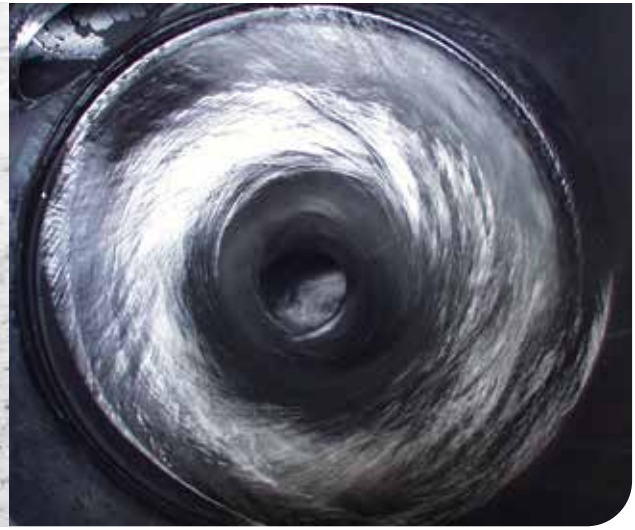
Flow characteristics in the energy dissipation chamber
