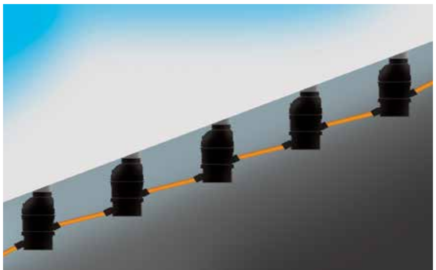
Principles of sewage system construction principle with the use of energy dissipating chambers
