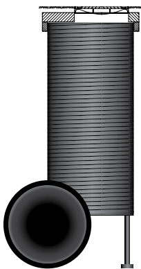
Figure 2. Example of a solution for an eccentric manhole made of structural pipes.
