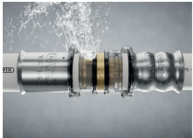
Fig. 31: Defined leak when testing with water.
