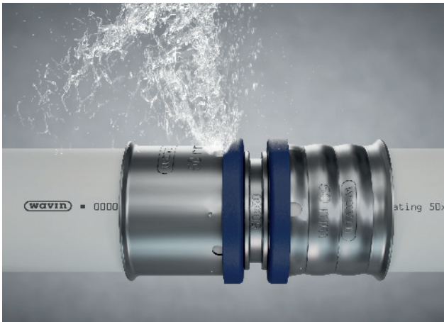
Fig. 16: DEFINED LEAK in the pressure test reveals with leaking water the unpressed fitting.
