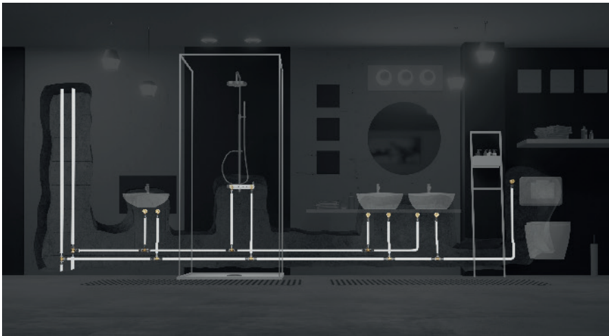
Fig. 42: Single Tee installation.
