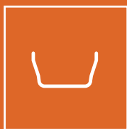
SquareLine 100mm (4") Square section gutter
