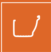
StormLine 111x76x97 (4¼x3¾") Ogee profile gutter
