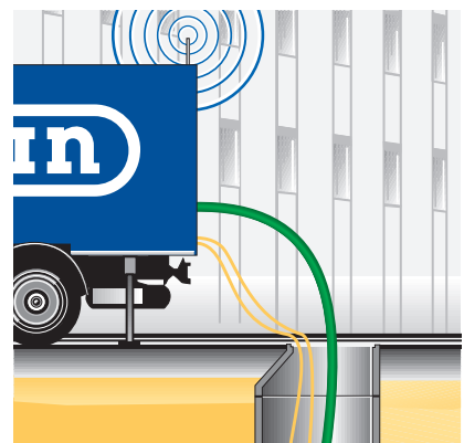
Fig. 3: Steam unit with integral process control
