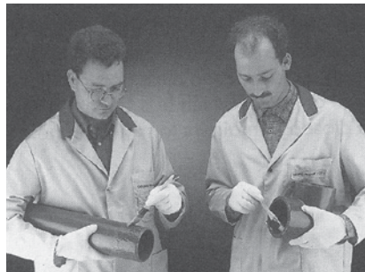
Solvent cement coat at d \geq 110 mm.
