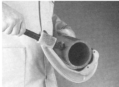
Cutting the pipe to length.
