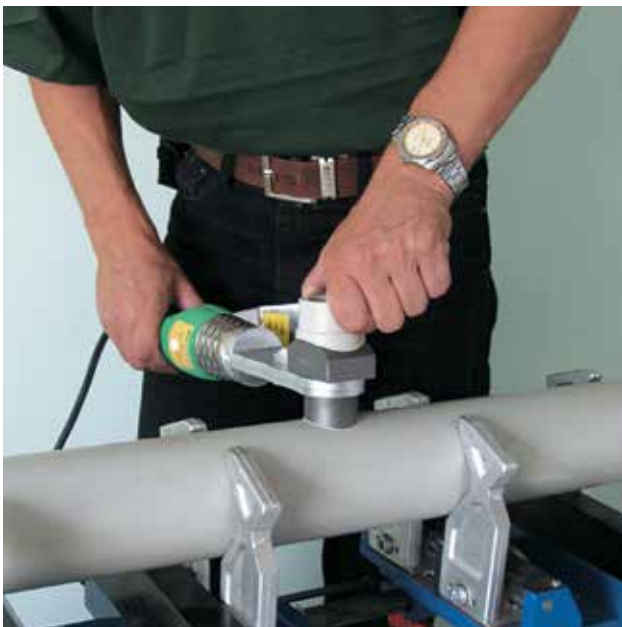
3. Put the plastic weld-in saddle on the adapter so that the mark on the saddle and the mark on the adapter are aligned. Heat-up the hole and the plastic weld-in saddle. The heating period is the same as with the 32 mm diameter (8 sec.). For weld-in saddle parts 110 × 32 and 110 × 40 the heating-up period is the same as for the 40 mm ones (12 sec.).
