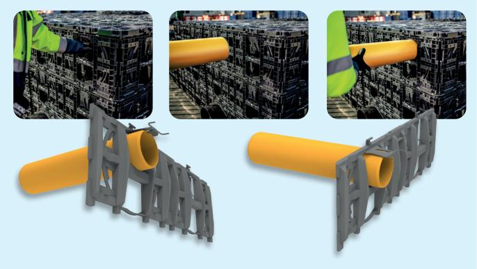
Step 9b Connection 160mm: Each side panel also has two preformed openings that can be cut by a jigsaw. Next, the Inlet connector with spigot DN200 and DN315 can be connected by positioning and rotating until clicked into place. (Bayonet like).
