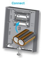
Open sensor and place batterie(s). Bat. Type: 3V CR123A 4 years (one battery), 10 years (two batteries)
