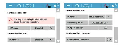
The Sentio device uses a dynamic IP address obtained via an DHCP request. If the IP address requires to be static for the network this can be achieved by configuring the applicable switch or router to serve a static IP address based on MAC address or hostname. The MAC address can be obtained via the sticker on the unit, the hostname used by the Sentio system is:
