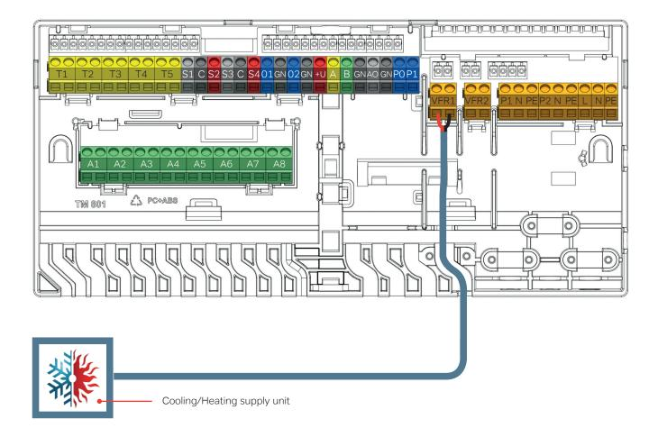
Connecting a heating or cooling source (example, depending on choosen profile).
