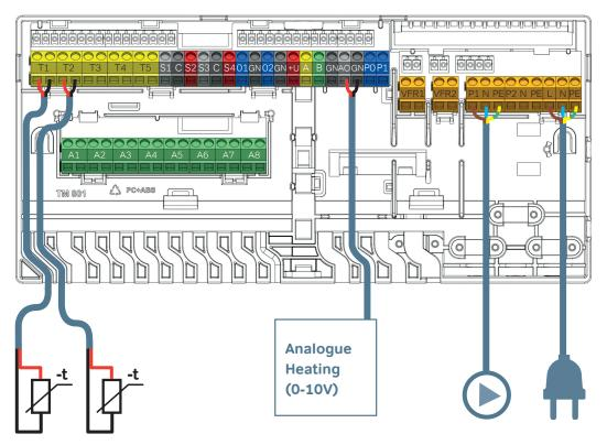
Connections Condensing Boiler.
