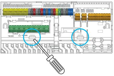
Demounting CCU and EUs from a DIN rail.
