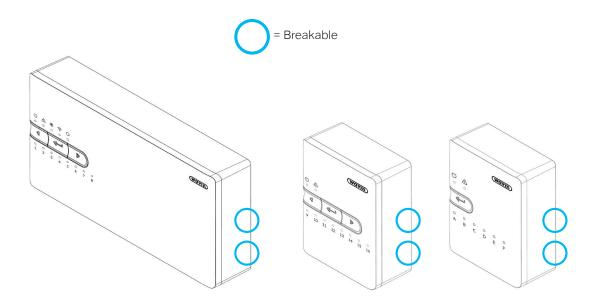
Breakable parts at the front plates when using interconnection cables.
