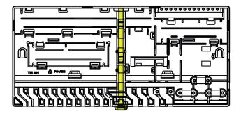
CCU back plate incl. locking-pin.
