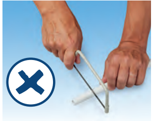
Figure 7: Don't use a hacksaw to cut Hep 2 O pipe
