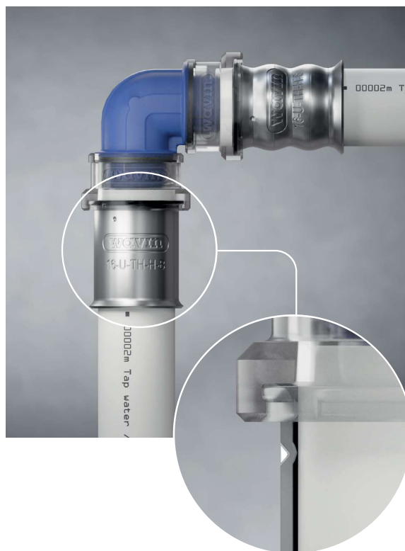
Fig. 15: PIPEGRIP. Firmly holds the pipe in position to have free hands for operating the pressing machine.
