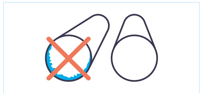
Figure 56: Before installation, pipes must be checked for damage and contamination
