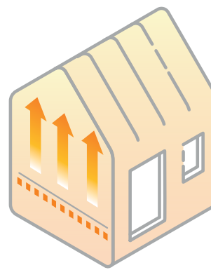
Fig. 2: Heat distribution in room with UFH.
