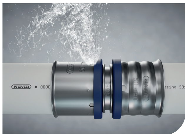
Fig. 9: DEFINED LEAK in the pressure test reveals with leaking water the unpressed fitting.
