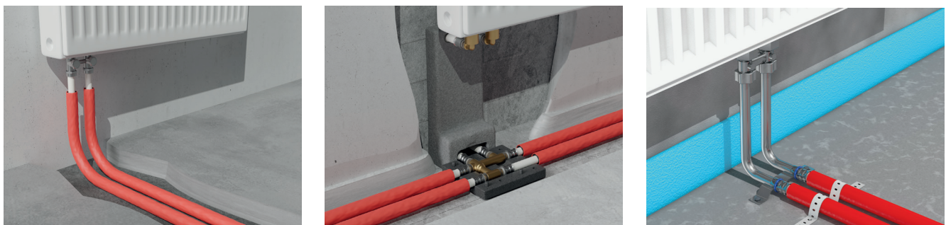
Fig. 45: Radiator installation examples with “Eurocone” screw connection.
