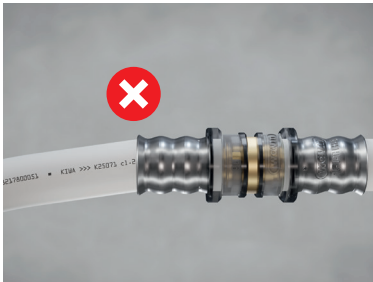
Fig. 25: Bending of the pipe directly at the fitting is not allowed. A minimum distance of 3 cm must be observed.
