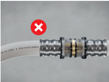
Fig. 25: Bending of the pipe directly at the fitting is not allowed. A minimum distance of 3 cm must be observed.
