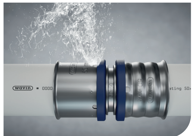
Fig. 18: DEFINED LEAK in the pressure test reveals with leaking water the unpressed fitting.
