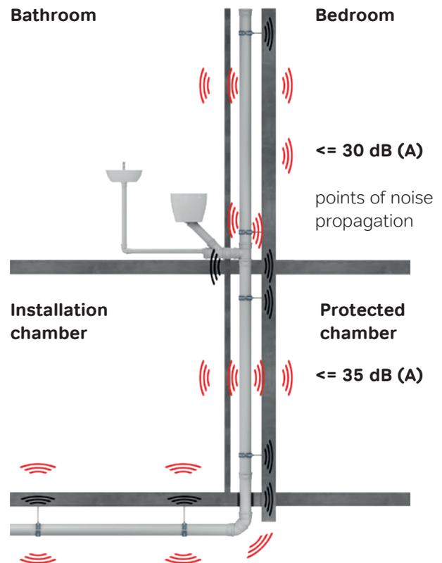
Fig. 5: Example of noise propagation during drainage.
