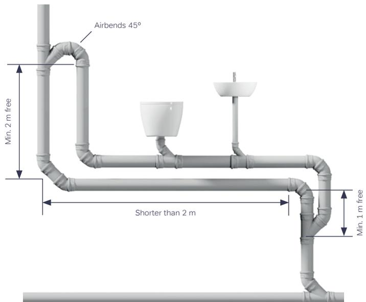
**Fig. 23:** Bypass pipe conforming to DIN 1986-100.
