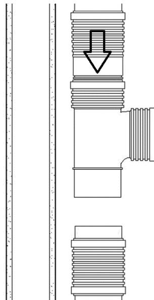
**11.** Slide the repair coupler over the spigot end of the branch or to the marking on the pipe.
