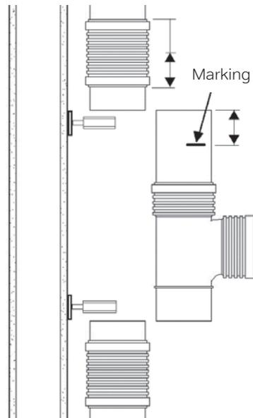
6. Install as close as possible to the two pipe ends wall plates for the fixed-point brackets and mount the threaded rod and back part of the brackets. When fixing the repair couplers with tensile resistant clamps this step can be skipped.
