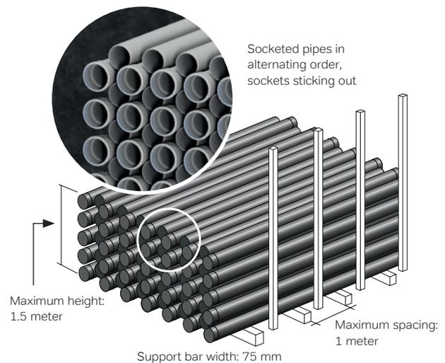
Stack pipes of different sizes separately or, if this is not possible, stack them in such a way that the largest diameter pipes are at the bottom. Pipes with sleeves should be stacked alternately so that they are supported along their entire length (see picture). Fittings are supplied in boxes and must be stored indoors. Do not subject fittings to heavy loads, as this can deform them.
