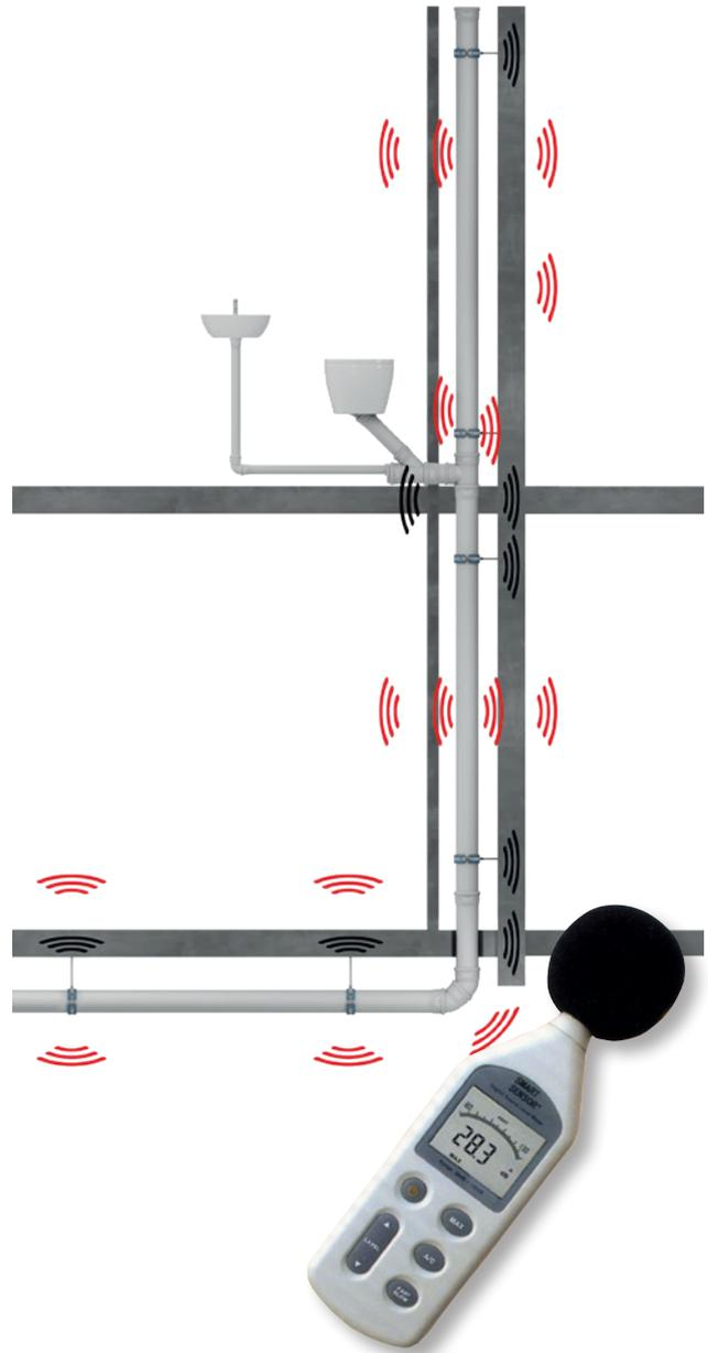
**Fig. 3:** FRAUNHOFER Test set up for determination of the installation sound level in the laboratory.
