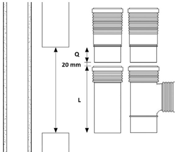
When replacing a piece of pipe, secure that the total length of the new socketed pipe (L) equals the length of the part cut out minus the length of the spigot of the branch (Q) minus 20 mm.
