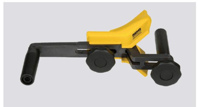
For connections to Wavin AS+ fittings or sockets the pipe end needs to be chamfered. Its is recommended to chamfer over a length of 5 mm under a 15 degrees angle. This can be done by using standard chamfer tooling.
