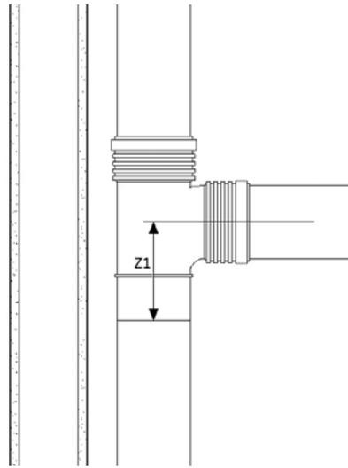
2. When inserting a branch, the length of the part to be cut out should have the length of the branch (L) + 20 mm + the length of the spigot of the long socket (Q).
