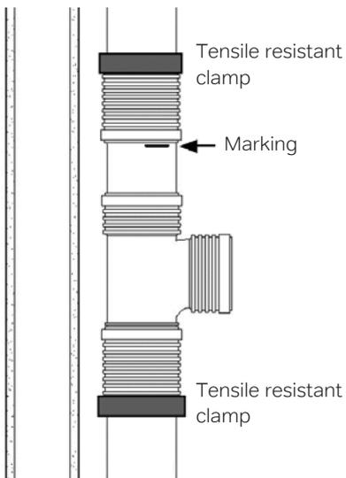
1. When inserting a branch at a later stage, please secure that the level of the branch is located at the right height. The Z1 value is mentioned for each branch in the product overview.
