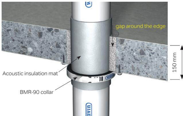
**Fig. 44:** Straight installation with / without sleeve / socket.
