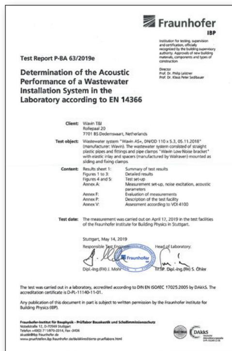
In studies conducted at the Fraunhofer Institut für Bauphysik (Fraunhofer Institute for Building Physics), Stuttgart, Wavin AS+ has proven its excellent sound absorption properties. The tests were performed in a laboratory accredited by the German Accreditation System for Testing (DAP, file no. PL-3743.26) according to standard EN ISO/IEC 17025.
