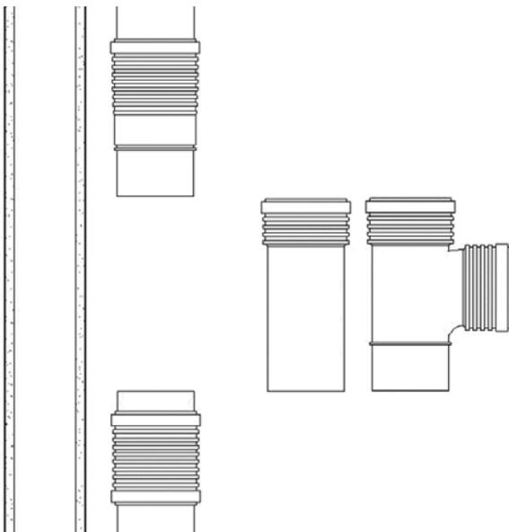
7. Push the socketed end of the branch or pipe on to the long socket.
