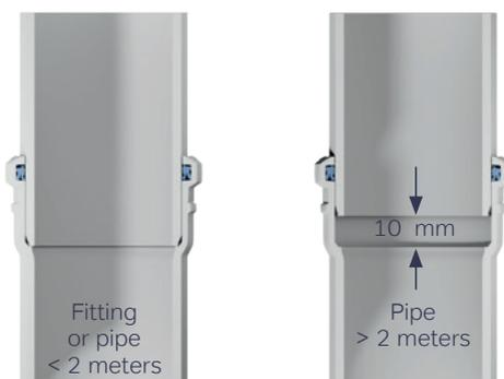
Fig. 27: 10 mm space for thermal expansion.
