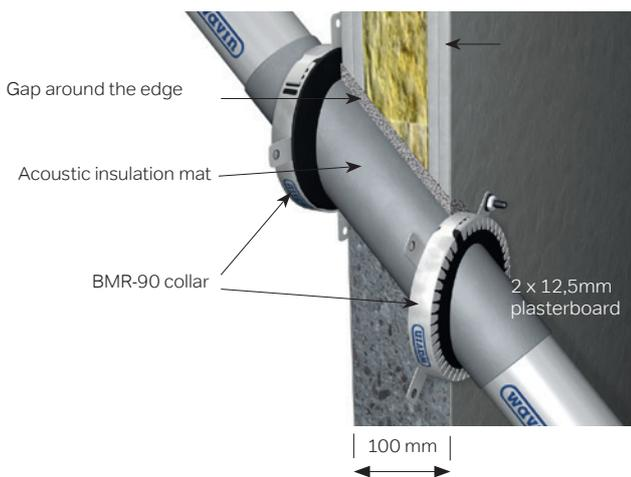
**Fig. 48:** 45° angled installation with / without sleeve / socket.
