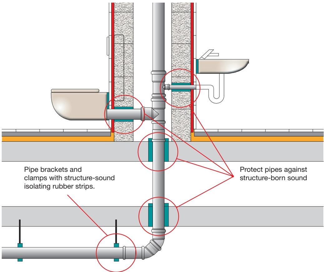
Fig. 9: Sound insulation of waste water systems.
