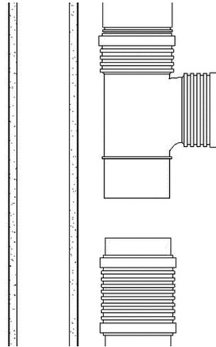
8. Push the long socket with the branch or pipe till the two pipe ends meet.
