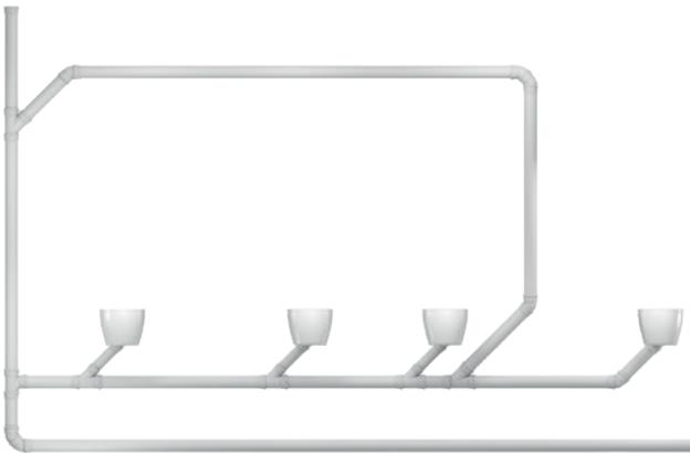
**Fig. 22:** Air-circulation pipe.
