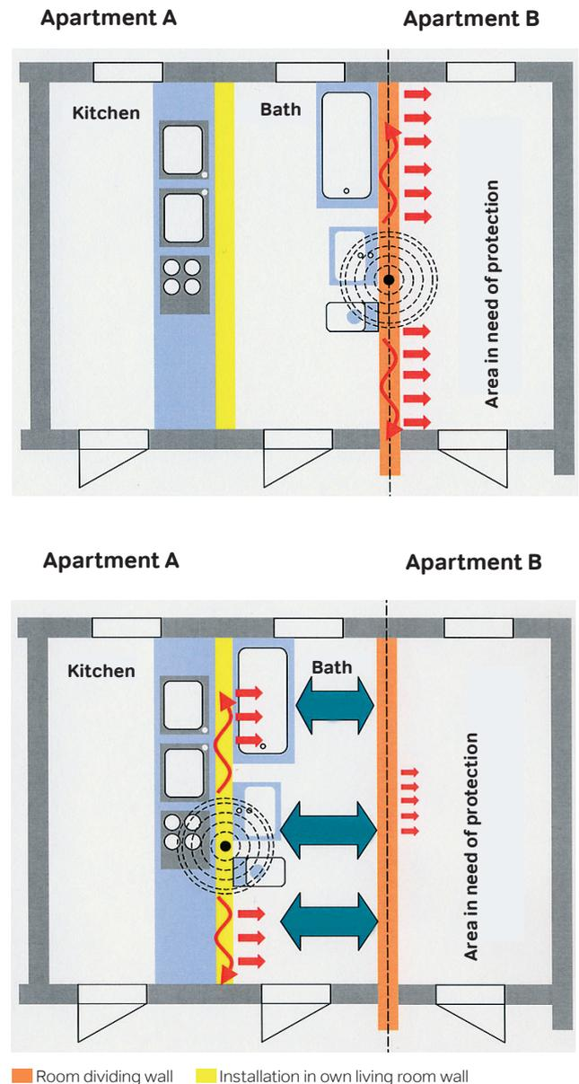
The comparison of the floor plans above demonstrates how good acoustic design in the lower building example can significantly reduce the noise levels to which areas requiring noise protection are exposed.
