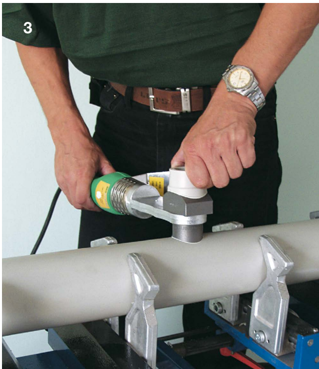
3 Put the plastic weld-in saddle on the adapter so that the mark on the saddle and the mark on the adapter are aligned. Heat-up the hole and the plastic weld-in saddle. The heating period is the same as with the 32 mm diameter (8 sec.). For weld-in saddle parts 110 x 32 and 110 x 40 the heating-up period is the same as for the 40 mm ones (12 sec.).
