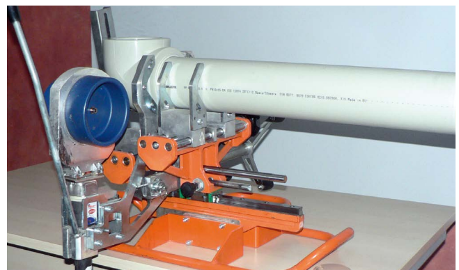
finished weld after the cool-down
