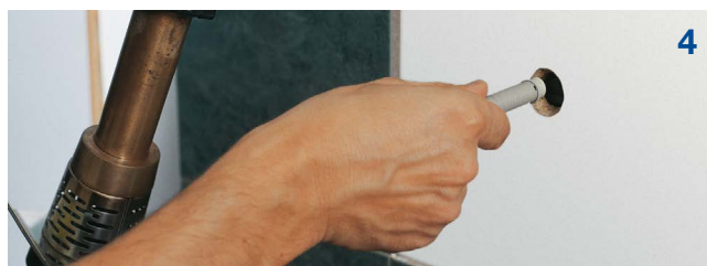
Take down the repairing stake and insert without turning into the heated hole.
