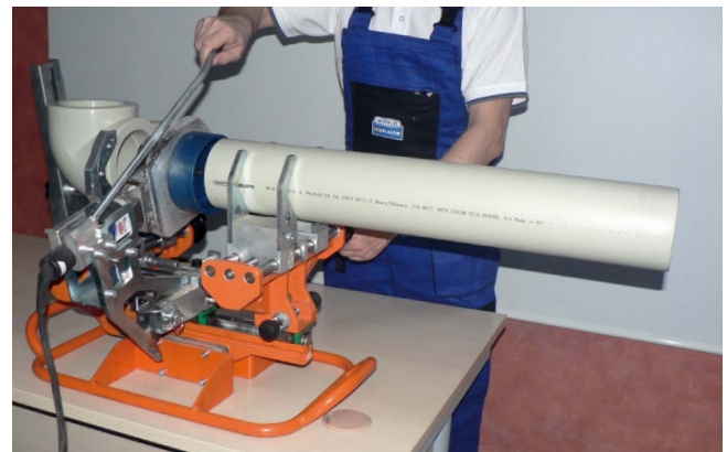
fixing and aligning the components, then heating them up
