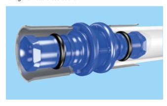
Figure 4: Safety through clever technology: the Defined Leak Function in the pressure test reveals unpressed fitting connections
