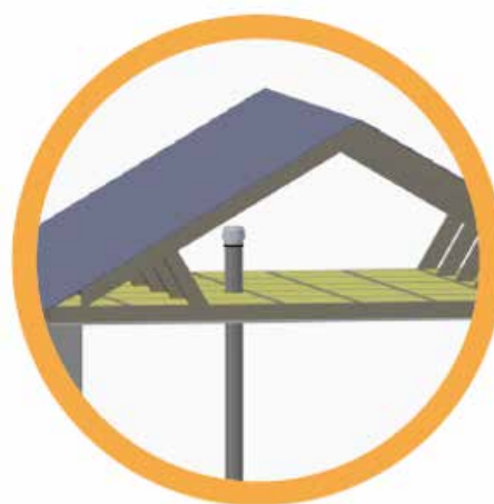
AAV terminating in roof space
