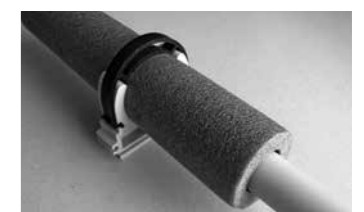
For hot water, the clip must be one size larger than the pipe (needs to be fitted over the insulation).
